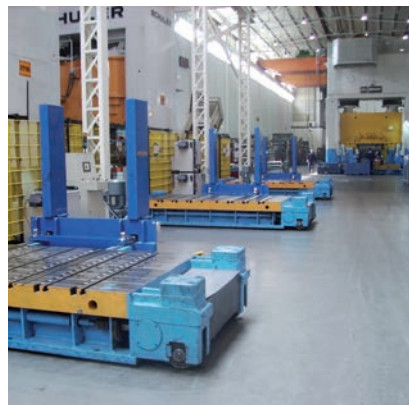
Push-pull system (PPS) for optimal positioning of the tool in the integrated press on the truck by the customer
