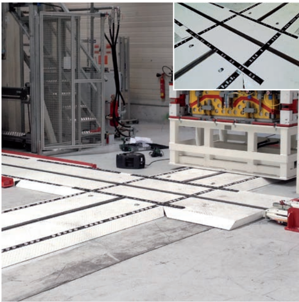
Quick Die Change system using rolling ramps
