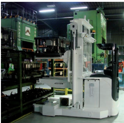
Driver-operated truck with dual load platforms for loading and transporting tools between presses and storage areas
