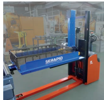
Basket carrier stacker for loading and unloading thermal ovens
